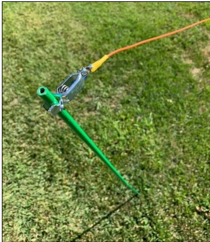
Figures 7-8: Elevated radial deployment with radial clip and 20M SWR measurement.
